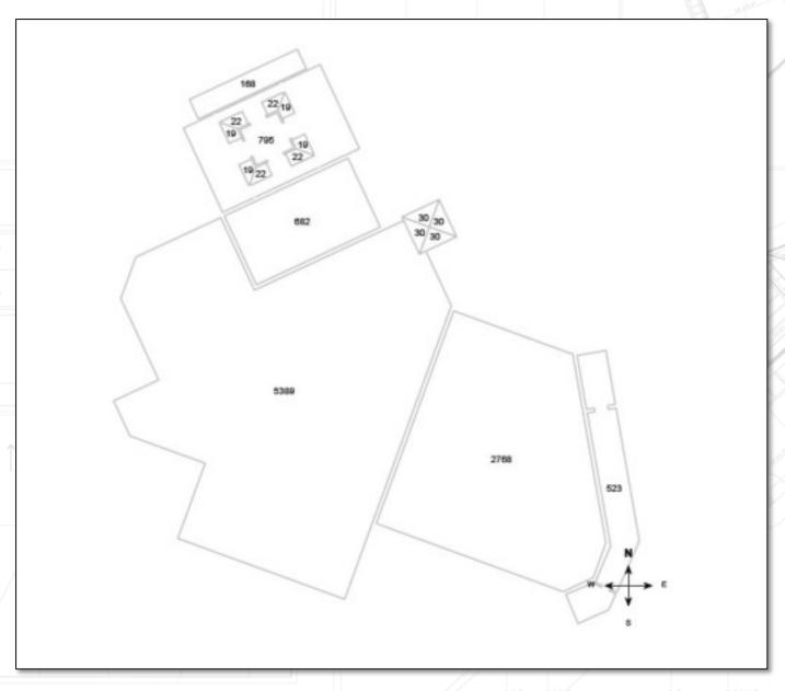
**Note:** This diagram shows the square feet of each roof facet (rounded to the nearest foot). The total area in square feet, at the top of this page, is based on the non-rounded values of each roof facet (rounded to the nearest square foot after being totaled).
