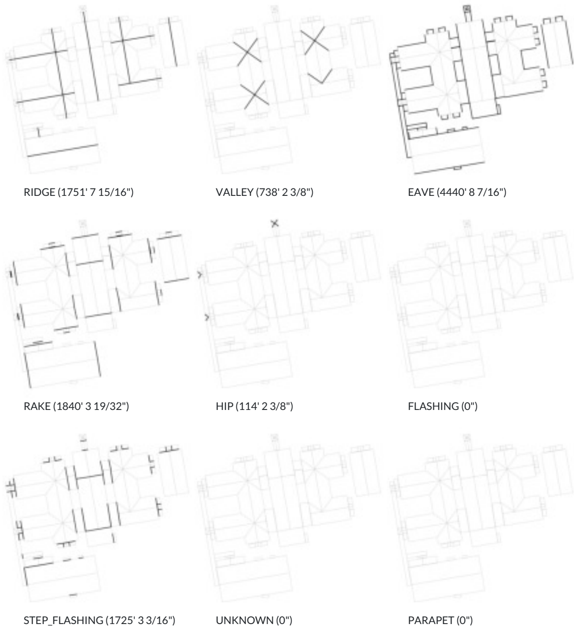
Figure 11: Roof Edge Classification (units: ffi)
